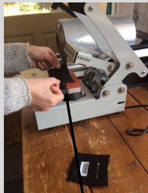
Place Label with barcode facing fabric with arrows up before Heat Seal Application of Label.
