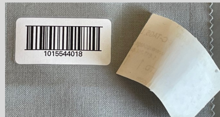
Place Label with barcode facing fabric with arrows up before Heat Seal Application of Label.
